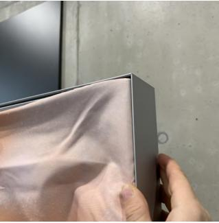
9b. **OPTIONAL** – Install the print for back (non-illuminated) in the outer sleeves the way that print covers the LED curtain. Follow instructions from the previous steps.
